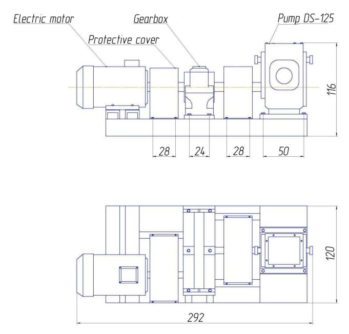
Figure 3 – Installation of bitumen pumping
