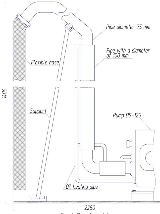
Figure 4 – Bitumen loading device
