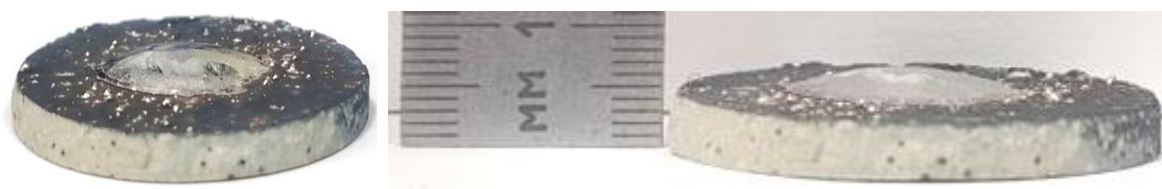
Figure 3. View of the sample after the experiment on the wettability of titanium melt on a BaZrO 3 substrate
