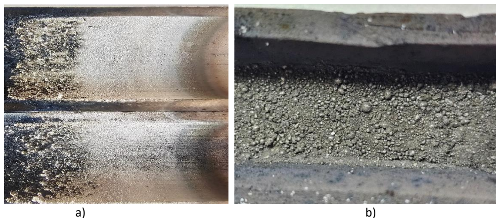
Figure 1. Magnesium condensate (a) and residue after distillation with spherical tin granules (b)
