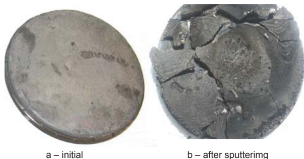
Figure 7 – Cobalt aluminide target destruction
