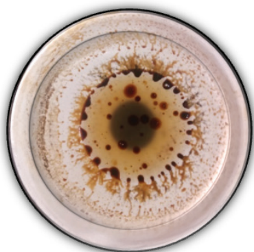
Figure 2 – The remaining phase after removing alcohol from the filtrate from slime washing
