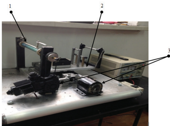
1 - winding core mandrel, 2 - movable carriage, 3 - electric motor
