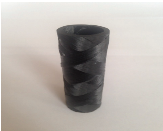
Figure 6 – CFTR from roving 24K with a cross-winding angle 45^\circ
