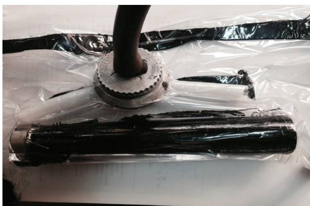
Figure 8 – Vacuuming process of the formed «raw» CFTR in a vacuum bag
