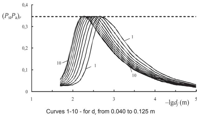
Figure 3 - Dependence of the combined effect of the steric and activation factors  $P_{st}P_a$  on the diameter of the rod  $d_r$  and grains  $d_j$
