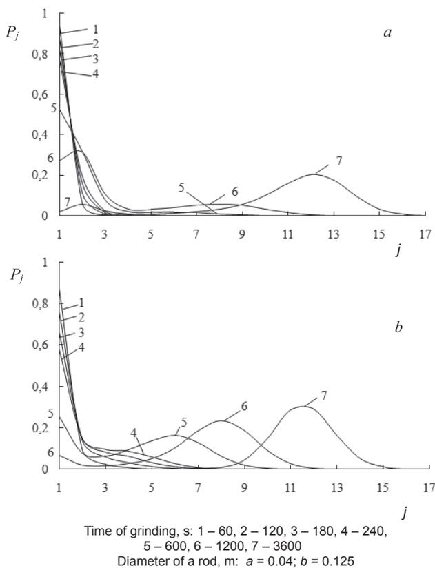
Figure 5 - Dependence of fractional composition ( $P_j$ , unit fr.) on the multiplicity of  $j$  and the time of grain grinding
