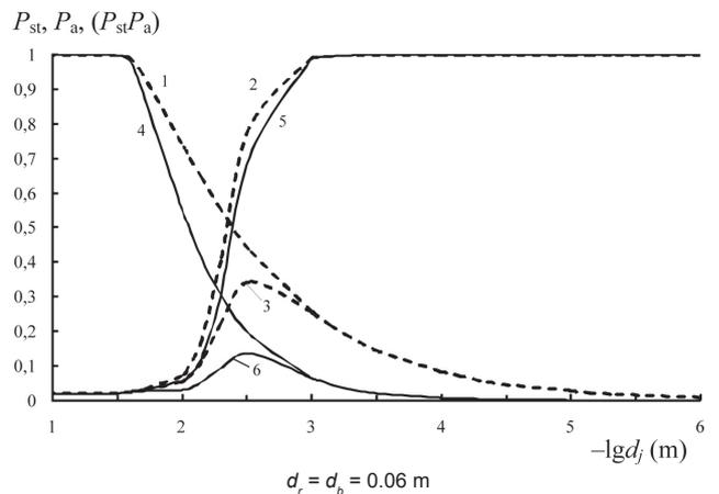
Figure 2 - Dependence of the steric (1, 4) and activation (2, 5) factors, as well as their products (3, 6) on the average size of the fractions for rod (1-3) and ball (4-6) grinding
