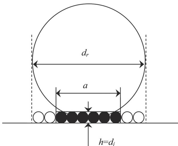
$d_r$  – rod diameter,  $d_j$  – grain diameter,  $h$  – circle segment arrow
