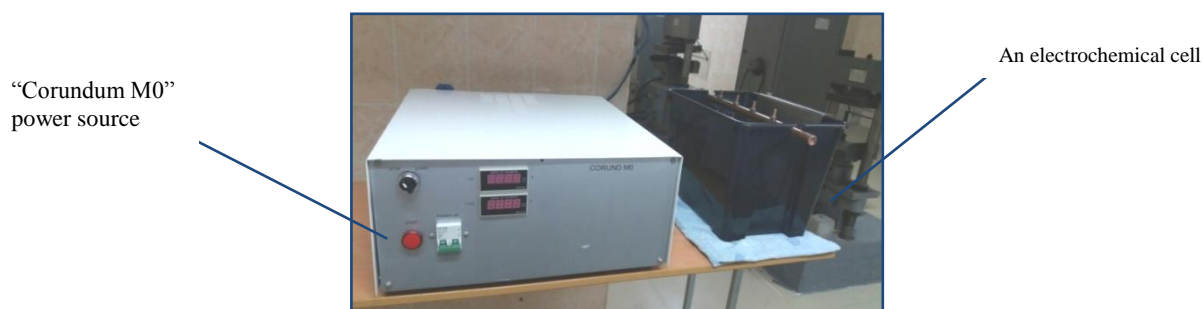
Figure 1 – An installation for modifying the titanium surface and its alloy
