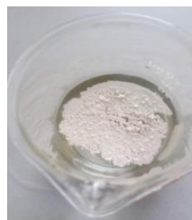
Figure 8 - Organoclay powder newly placed on the surface of the water after t=150 days
