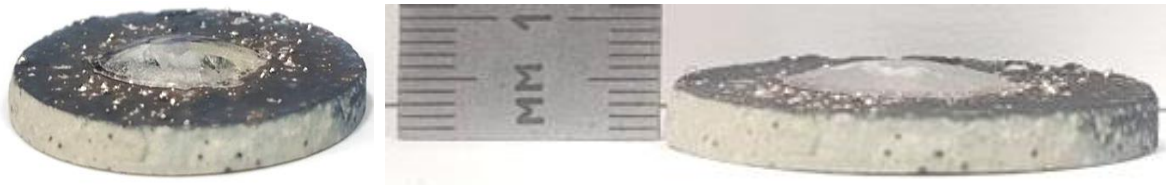
Figure 3. View of the sample after the experiment on the wettability of titanium melt on a BaZrO 3 substrate
