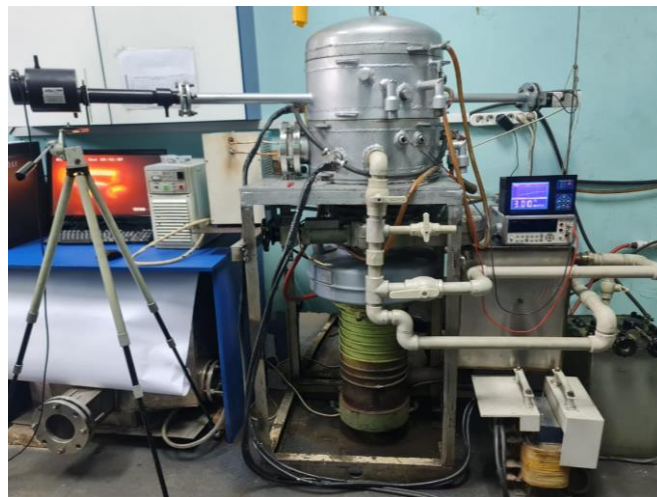
Figure 1. External view of the installation for determining the contact angle under high vacuum conditions
