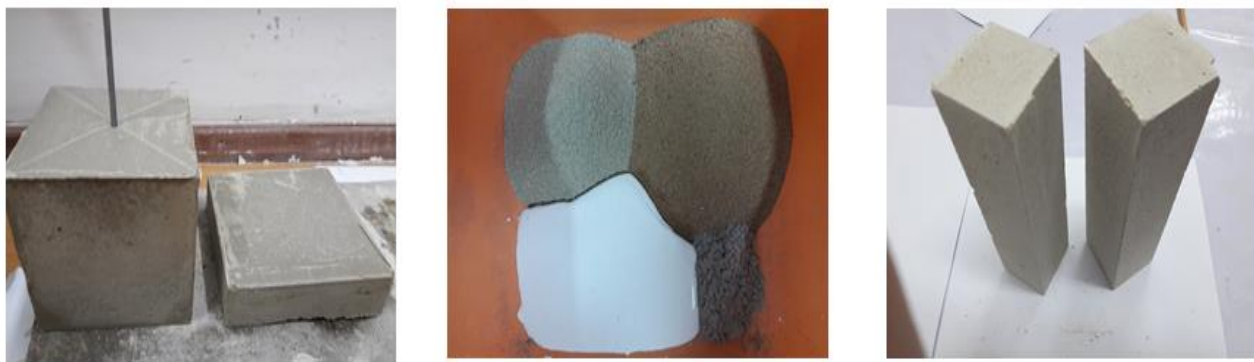
Figure 4. Samples of construction materials obtained using diatomite
