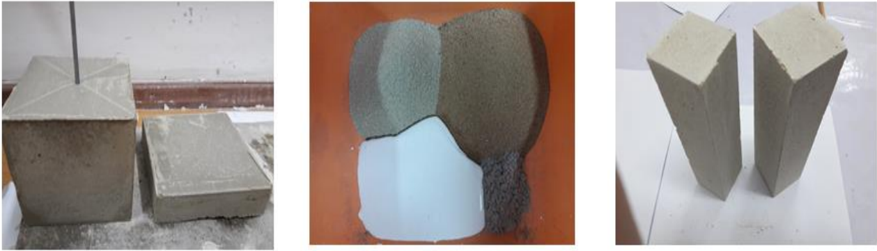
Figure 4. Samples of construction materials obtained using diatomite
