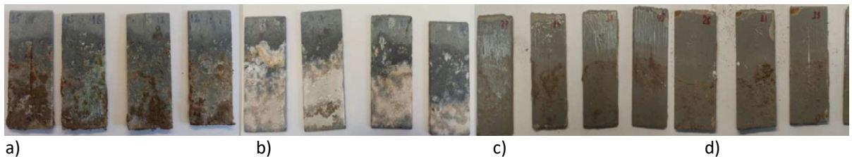
Figure 4. View of samples after testing on the “Laboratory installation for modeling pipeline transport technologies”: Samples with CLP: a) without ECP; b) with ECP. Samples with two-component EPLP: c) without ECP; d) with ECP
