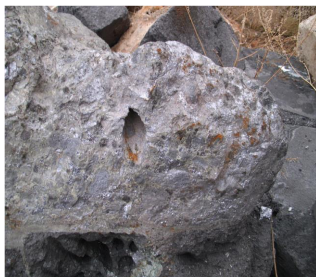
Figure 4 - Photo of the furnace encrustation pieces – Slag-carborundum from the "frozen" furnace
