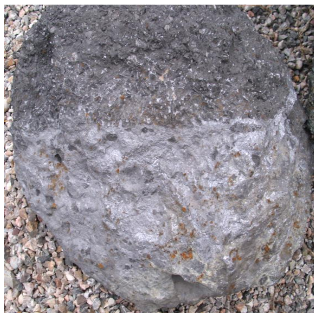
Figure 1 - Photo of the frozen part of the charge and the furnace encrustation in an industrial arc furnace: crystallized mixture of silicon carbide with inclusions of silicon and quartzite (silicon oxides) reduced by 20 times M1:20
