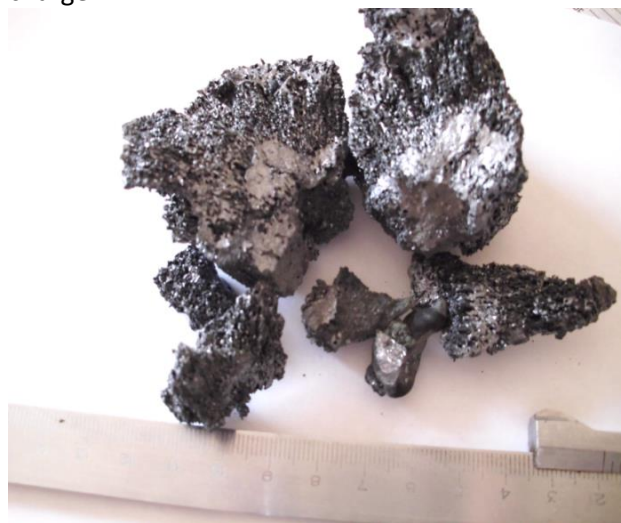
Figure 3 - Quartzite coated with silicon carbide during silicon carbothermy in an electric arc furnace
