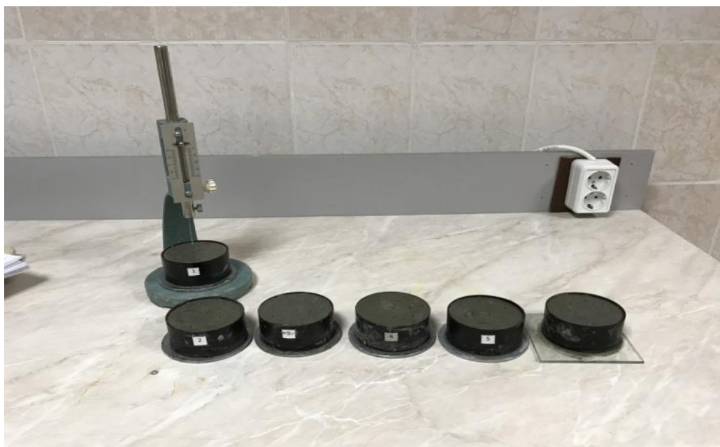
Figure 1 – Determination of the setting time of the cement paste on the Vica device
