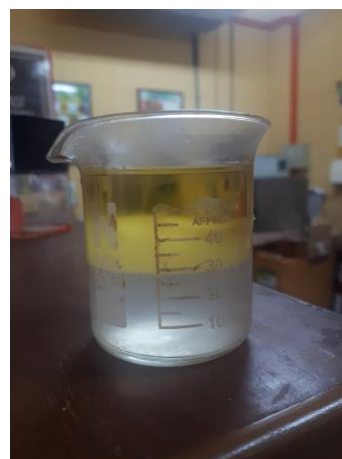
Figure 4 – End of oil-water emulsion demulsification process by grafted copolymer
