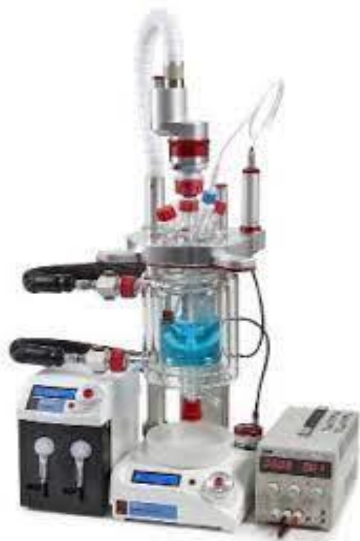
Figure 1 – Syrris Globe reactor used for synthesis with doser
