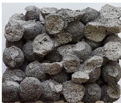
Figure 6 – The nature of destruction of the composite material during the strength test
