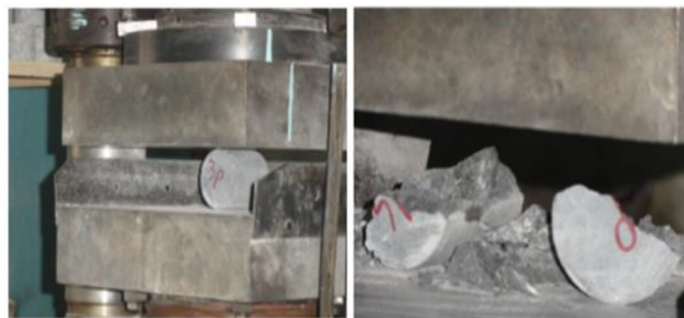
Figure 2 - Testing of rocks for tensile strength under uniaxial tension
