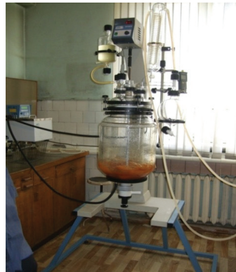
Figure 1 – Image of pilot installation (R-620) (Selecta, Spain) for synthesis of flotation reagents
