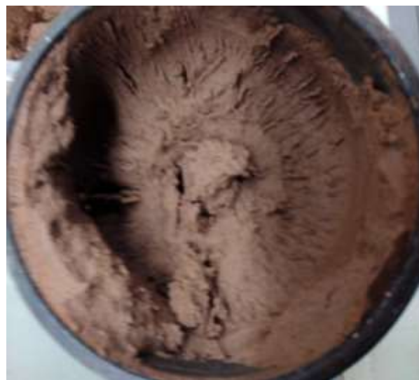
Figure 4 - Solid phase of bauxite activation. obtained at 200 ° C and duration 90 minutes
