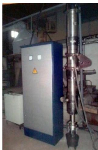
Figure 2 - Experimental sample of a mud-pulse gun
