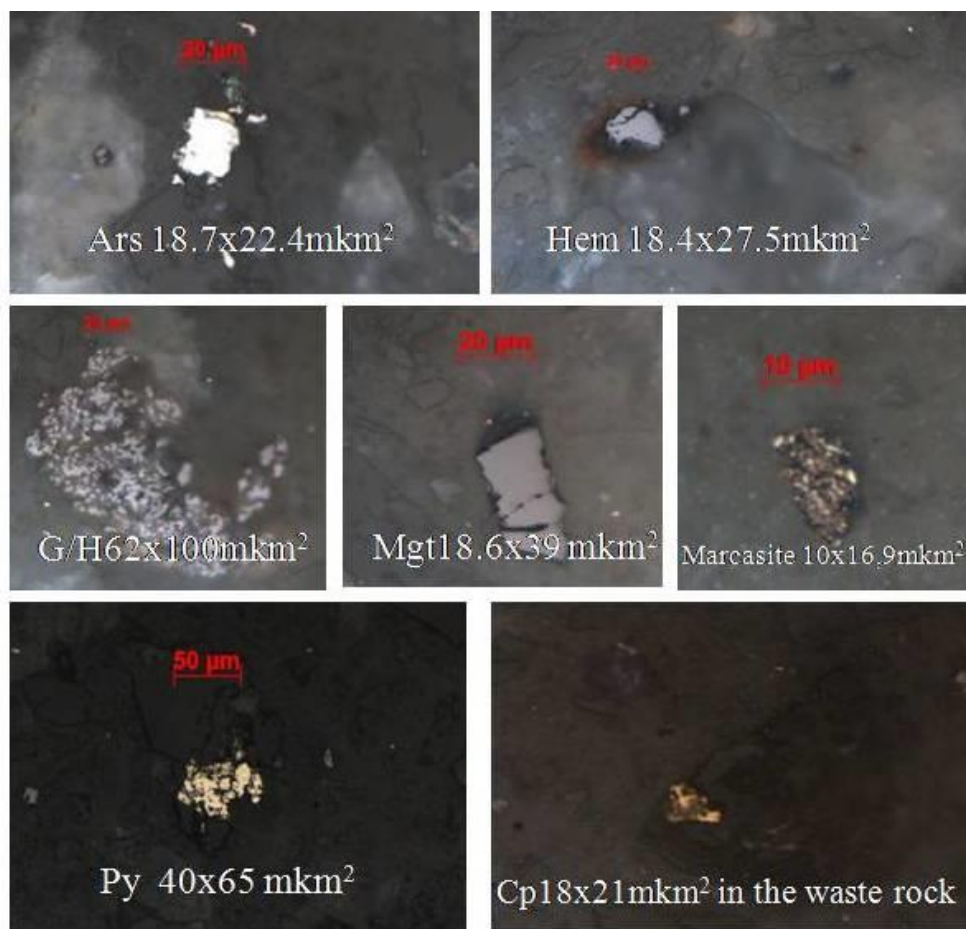
Figure 2 Finely dispersed gold in association with waste rock and bismuthin
