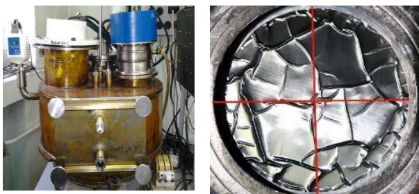
Figure 8 Upgraded chamber of the magnetron sputtering installation and the surface of the membrane of tantalum and niobium foil
