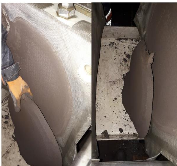
Figure 7 Photograph of a chromium-containing sludge cake from a pilot filter press
