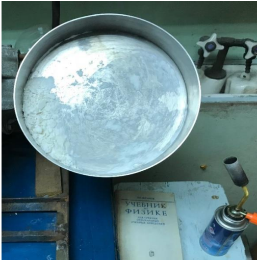
Figure 6 - Obtaining flake calcium nitrate using a granulator
