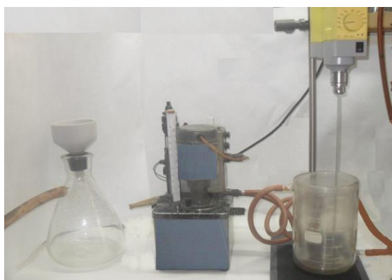
Figure 1 - Laboratory setup for Ni-Co concentrate deposition
