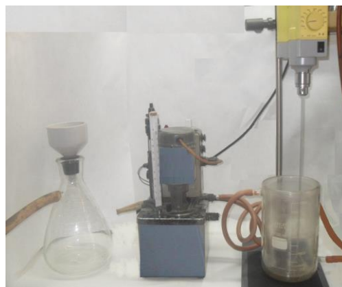
Figure 1 - Laboratory setup for Ni-Co concentrate deposition
