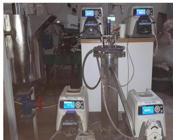
**Figure 3** Outotec laboratory thickener 99 mm in diameter
