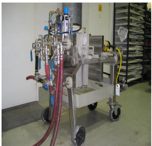
**Figure 6** Outotec pilot filter press with  $0.27 \text{ m}^2$  filtration area.
