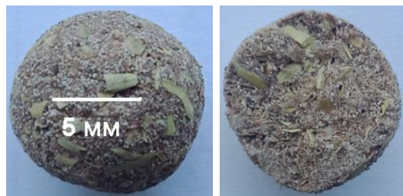
Figure 3 - Magnesia granule with combined filler
