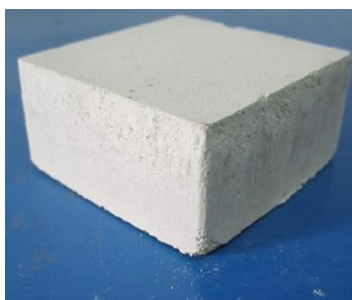
Figure 5 Pellets look after carbonization for 12 hours
