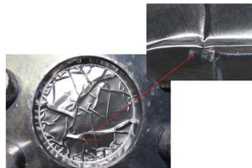
Figure 2 – Formation of a crack in hydrogen permeable membranes as a result of dilatation
