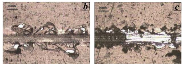
Figure 7 - Dependences of AE and CR (7a) CP coatings with a thickness of  $1.6 \mu\text{m}$  and surface micrographs at a load of  $F = 0.54$  N (7b) and  $F = 0.81$  N (7c)
